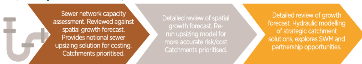
Figure 4-2: Summary of the sewer catchment capacity assessment process (Source: Anglian Water WRLTMP, Ref. 50)
