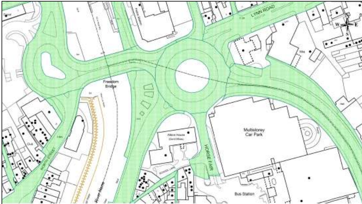
Figure 2.22: Highway Boundary Plan for Freedom Bridge Roundabout
