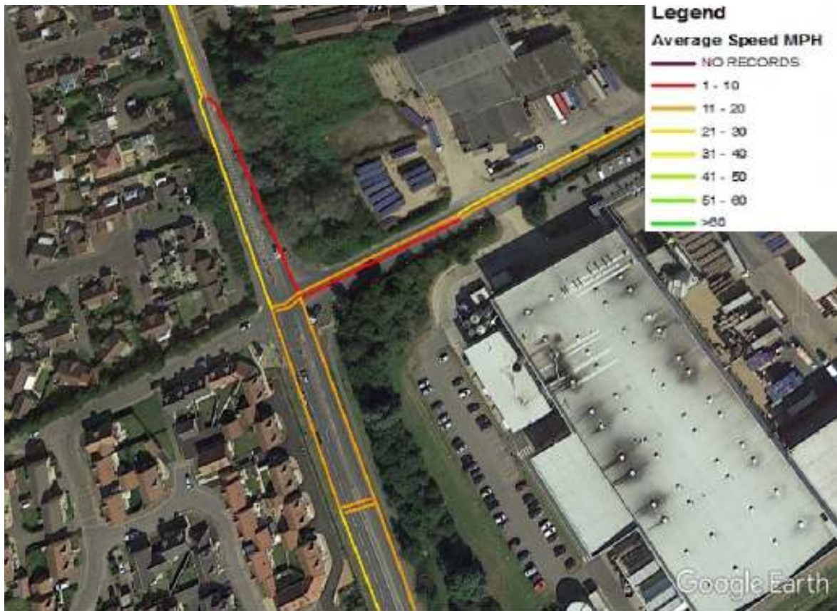
Figure 2.26: Cromwell Road / Weasenham Lane Junction Average Speed PM Peak Hour (17:00 - 18:00)
