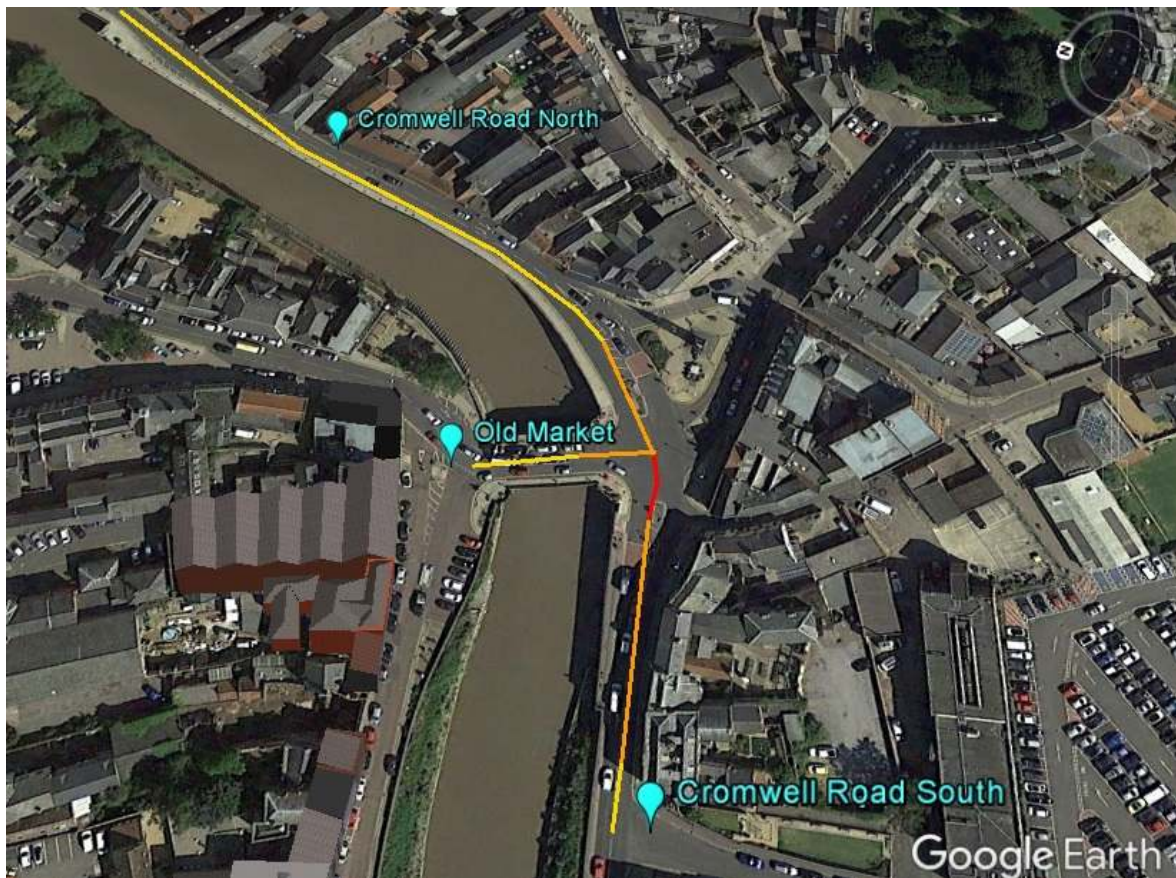
Figure 2.11: Town Bridge Junction TomTom Segments used per Approach
