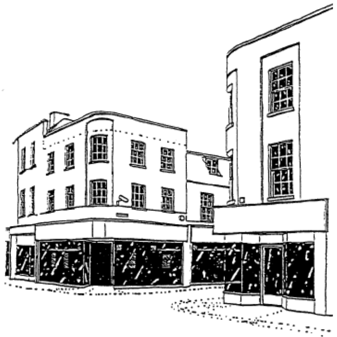
The effects of modern facias and plate glass on an old building
