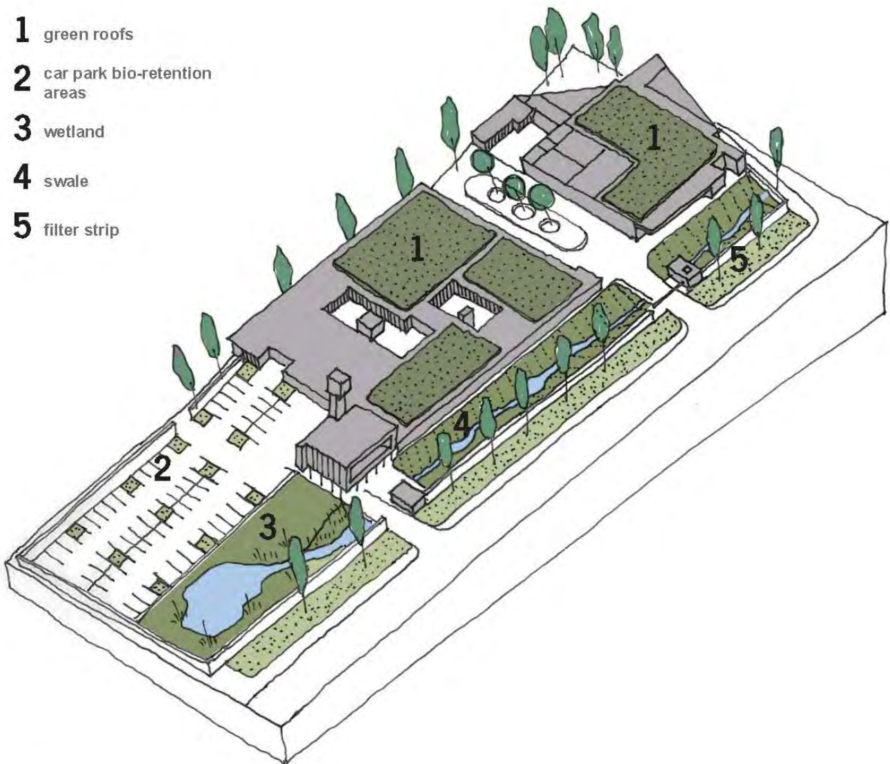
Figure 6.18 : Incorporating SuDS on industrial sites
